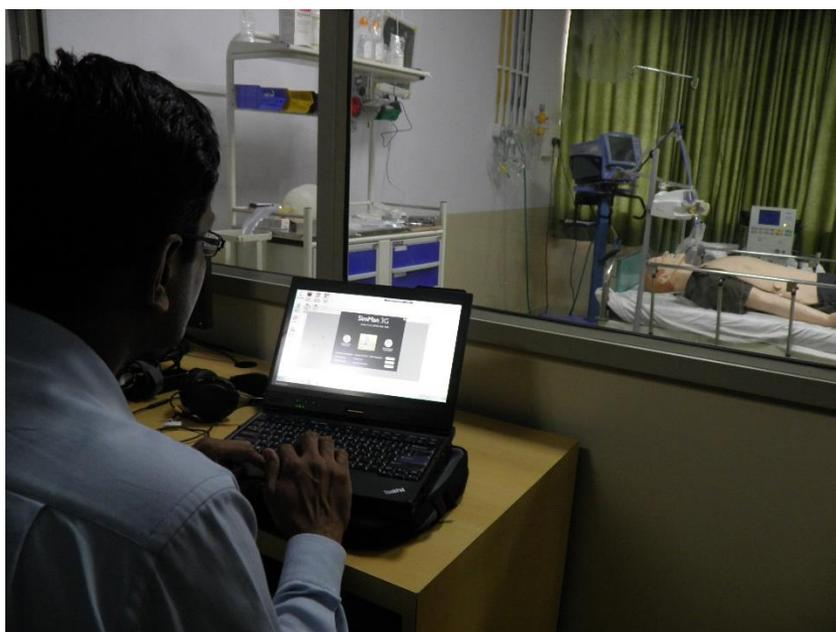
4. WLAN Communication System with Webcam: communication between these 3 units can be set up to wireless WLAN network. With the help of this system, the simulation lab is connected to a debriefing classroom via a camera which can transmit the simulation training live to other students.
